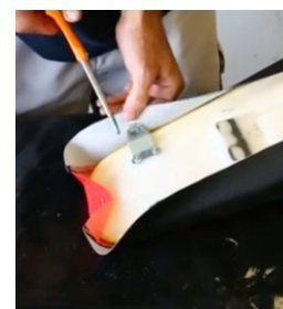
5 - Trim the cover around the seat mount area.
